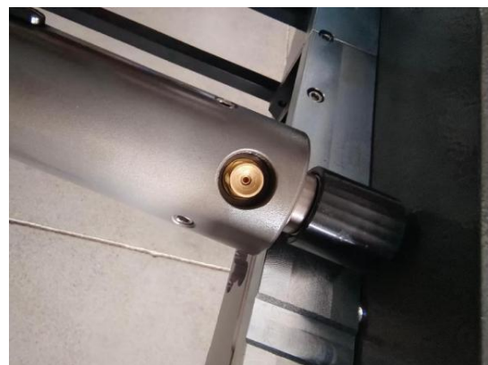
(2) 充气口/Air inlet position
